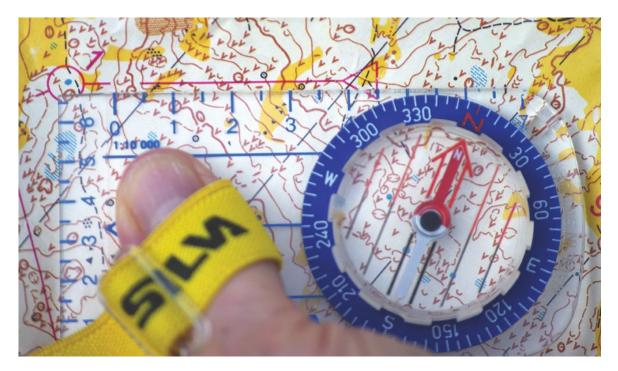
2. Rotate the bezel until the lines on the bezel are lined up with the north lines on the map
